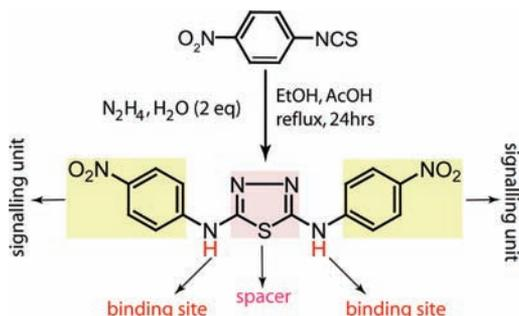
characterized by NMR, ESI-MS, UV-vis, and IR spectroscopies. The receptor  $\text{LH}_2$  consists of two acidic N–H protons which are separated by a rigid thiadiazole spacer. The 4-nitro phenyl rings help to increase the acidity of N–H protons and also act as a chromophoric signaling unit during the receptor–halide interaction process.
